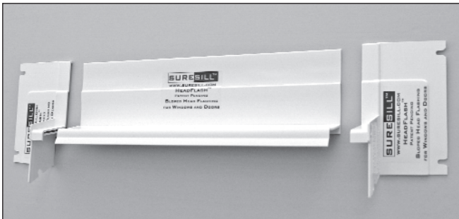
Figure 5. HeadFlash, a window drip cap made from rigid PVC, comes in three sections. The center section is first trimmed to length, and then the end caps are attached with PVC cement to form watertight joints.
